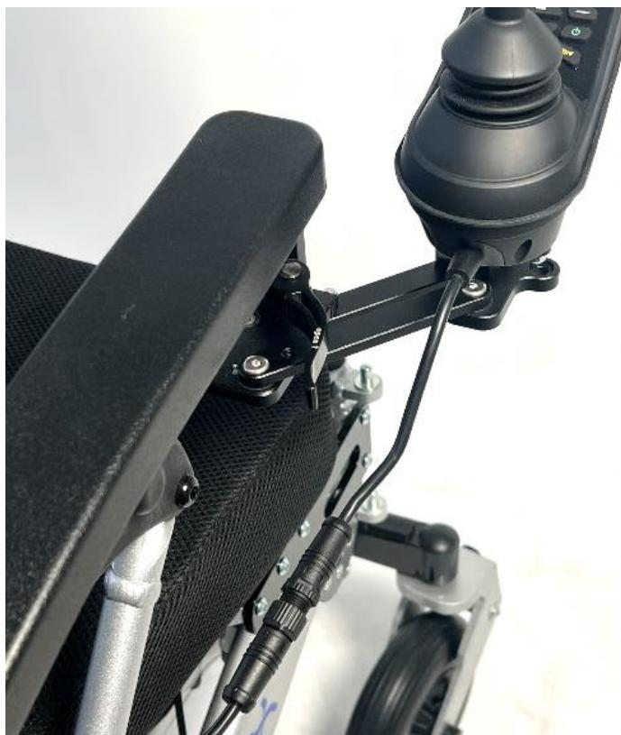
2. Attach the joystick mount onto the armrest as normal, making sure the cable runs smoothly on the outside with enough slack to allow the joystick to move freely.
